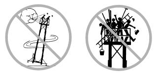
Occupants, equipment and materials shall not exceed the maximum platform capacity.
