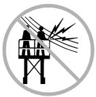
Keep away from the machine if it contacts energized power lines or becomes electrically charged. Personnel on the ground or in the platform must not touch or operate the machine until the energized power lines are shut off.
